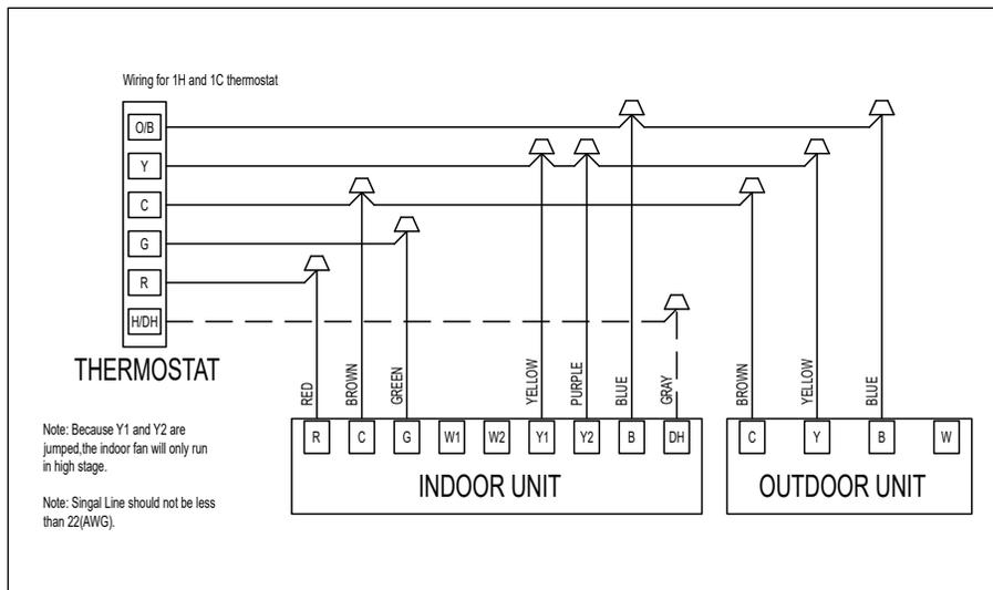
Figure 5 Control Wiring For 18SEER HP Systems
