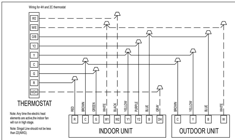
Figure 2 Control Wiring For 18SEER HP Systems
