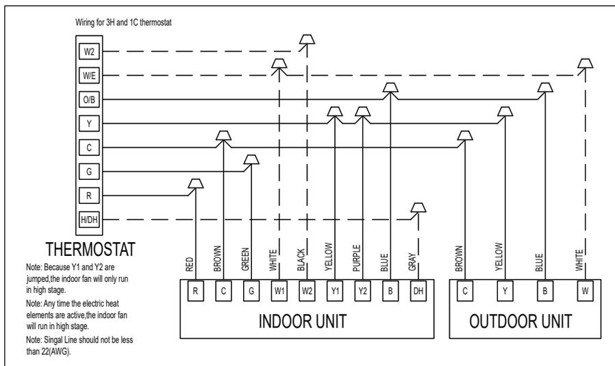
Figure 3 Control Wiring For 18SEER HP Systems
