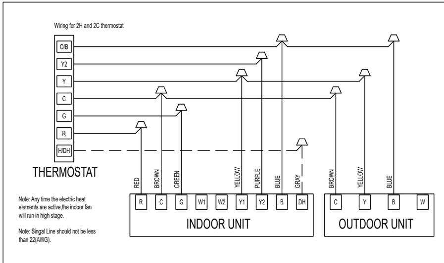
Figure 4 Control Wiring For 18SEER HP Systems
