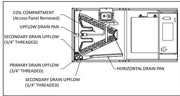
FIGURE 7: Coil Assembly
