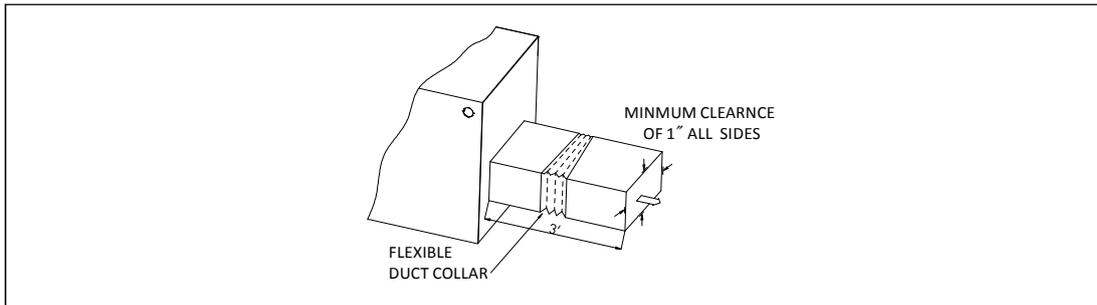
FIGURE 3: Dimensions and Duct Sizes
