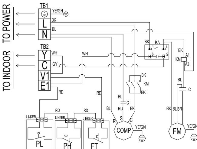
**Suggestion:** The wire diagram is as FIGURE 10 when the outdoor unit is getting feedback from terminals E1, V1.
